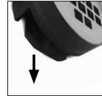
Let the cover slide out together with the batteries.
